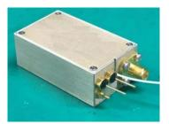
This product directly modulates the intensity of the laser in response to an input RF signal of 0.1-18 GHz, completing the electro-optic conversion. It outputs an RF-modulated optical signal at either the 1310 nm or 1550 nm Wavelength series. After transmission through an optical fiber, it provides a modulated optical signal to the optoelectronic conversion component (photodetector)
